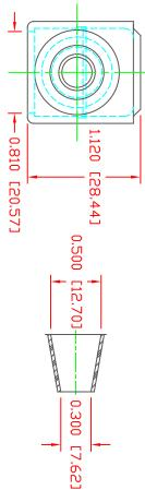
SECTION A-A TYP, WALL THICKNESS = .071" [1.800] SEAL NO. 2 SHOWN
