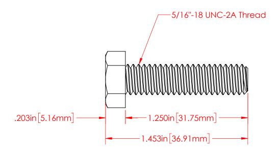
P/N 3730-000 5/16"-18 Fully Threaded 304 Stainless Steel Bolt
