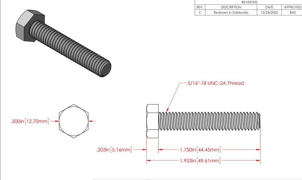
P/N 3730-001 5/16"-18 Fully Threaded 18-8 Stainless Steel Bolt
