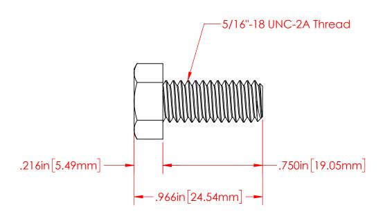
P/N 3730-006 5/16"-18 Fully Threaded 18-8 Stainless Steel Bolt
