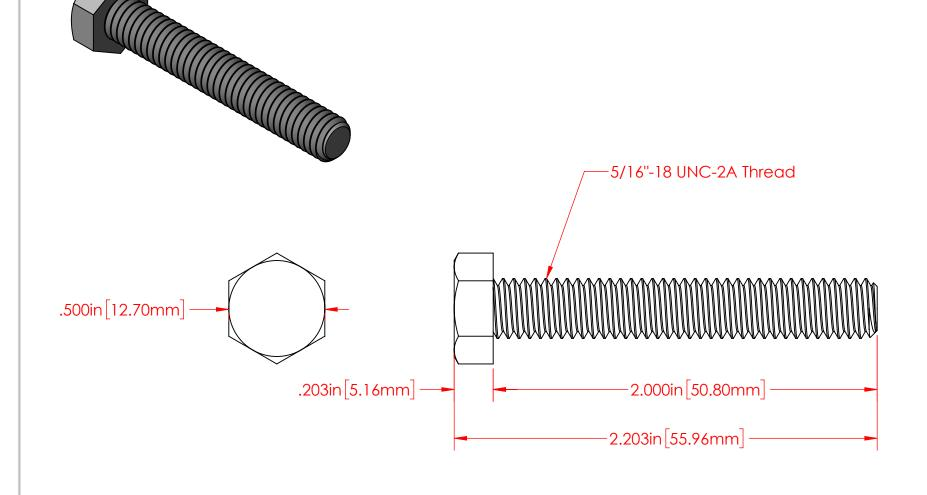
P/N 3730-007 5/16"-18 Fully Threaded 18-8 Stainless Steel Bolt
