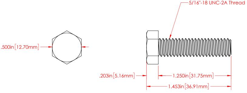
P/N 3730-010 5/16"-18 Fully Threaded Zinc Plated Mild Steel Bolt
