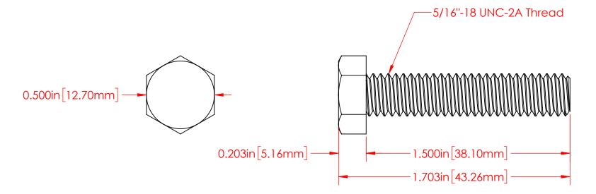
P/N 3730-011 5/16"-18 Fully Threaded 18-8 Stainless Steel Bolt
