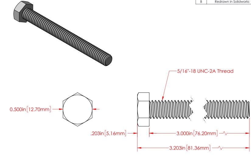
P/N 3730-012 5/16"-18 Fully Threaded 18-8 Stainless Steel Bolt
