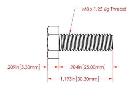
P/N 3731-000 M8 x 1.25 Fully Threaded 18-8 Stainless Steel Bolt
