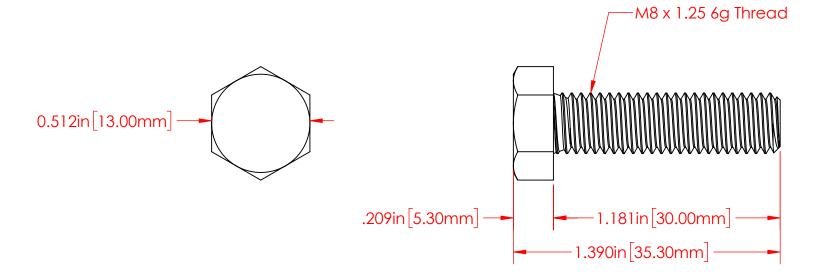
P/N 3731-001 M8 x 1.25 Fully Threaded 18-8 Stainless Steel Bolt
