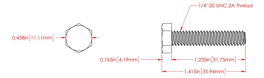
P/N 3736-000 1/4"-20 Fully Threaded 18-8 Stainless Steel Bolt
