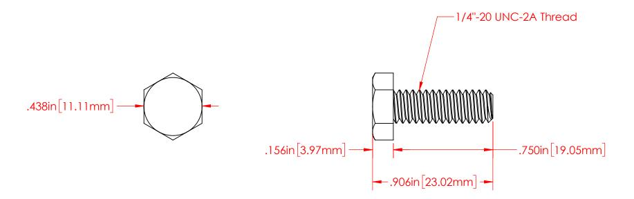
P/N 3736-003 1/4"-20 Fully Threaded 18-8 Stainless Steel Bolt
