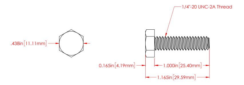
P/N 3736-003 1/4"-20 Fully Threaded 18-8 Stainless Steel Bolt
