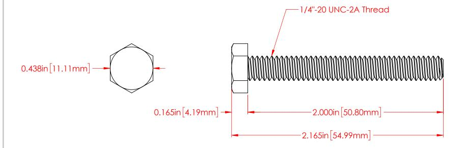
P/N 3736-004 1/4"-20 Fully Threaded 18-8 Stainless Steel Bolt
