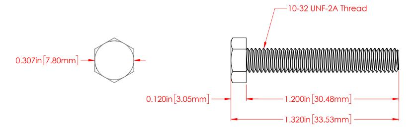
P/N 3737-000 10-32 Fully Threaded 18-8 Stainless Steel Bolt
