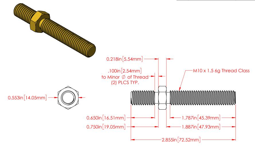
P/N 3739-003 360 Brass Alloy Double Ended Stud M10 x 1.5 Threaded Both Ends
