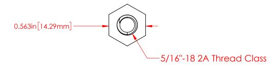
P/N 3739-005 Nickel Plated 360 Brass Alloy Double Ended Stud 5/16"-18 Threaded Both ends
