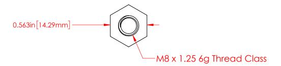
P/N 3739-006 Nickel Plated 360 Brass Alloy Double Ended Stud M8 X 1.25 Threaded Both ends
