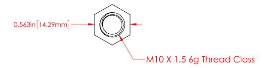
P/N 3739-008 Nickel Plated 360 Brass Alloy Double Ended Stud M10 X 1.5 Threaded Both ends
