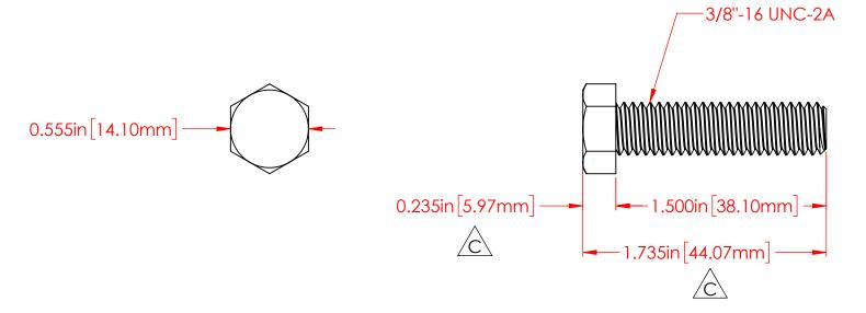
P/N 3740-001 3/8"-16 Fully Threaded 18-8 Stainless Steel Bolt
