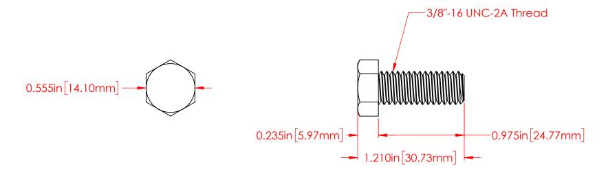
P/N 3740-006 3/8"-16 Fully Threaded 18-8 Stainless Steel Bolt
