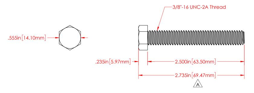
P/N 3740-008 3/8"-16 Fully Threaded 18-8 Stainless Steel Bolt
