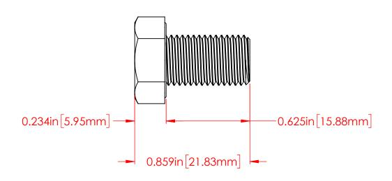
P/N 3740-011 3/8"-24 Fully Threaded 18-8 Stainless Steel Bolt
