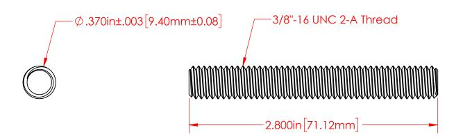
P/N 3742-012 3/8"-16 Threaded Stud Nickel Plated Mild Steel
