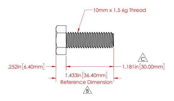
P/N 3743-000 M10 x 1.5 Fully Threaded 18-8 Stainless Steel Bolt
