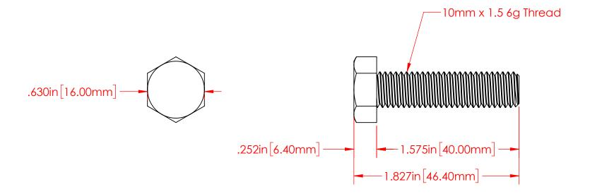
P/N 3743-001 M10 x 1.5 Fully Threaded 18-8 Stainless Steel Bolt
