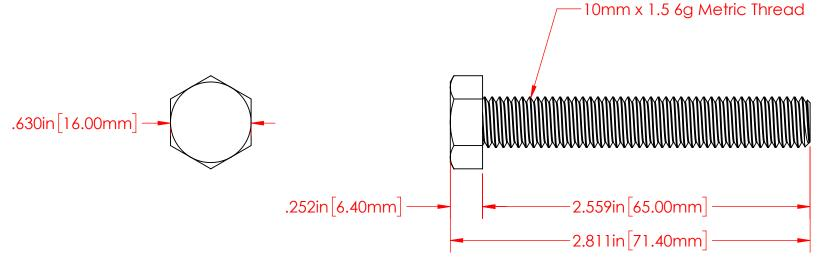
P/N 3743-002 M10 x 1.5 Fully Threaded 18-8 Stainless Steel Bolt
