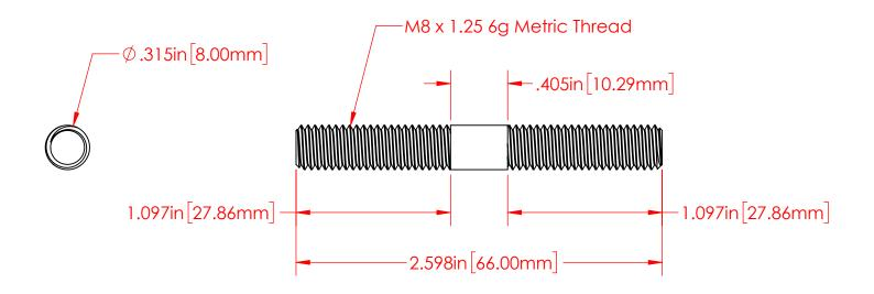
P/N 3744-003 M8 x 1.25 Threaded Stud Nickel Plated 360 Brass Alloy
