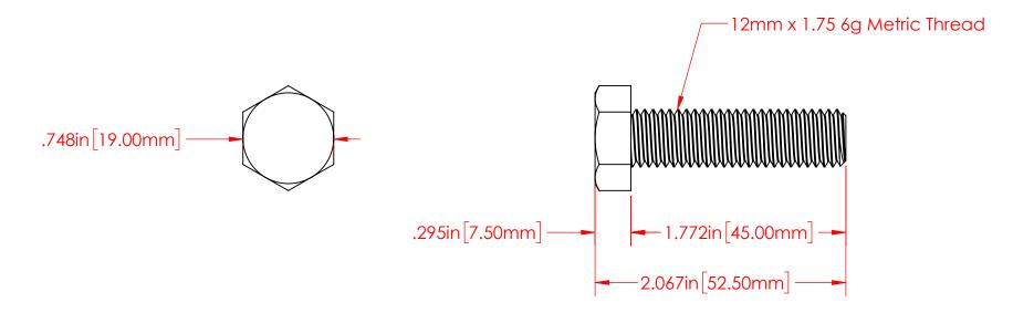
P/N 3746-000 M12 x 1.75 Fully Threaded Bolt 18-8 Stainless Steel
