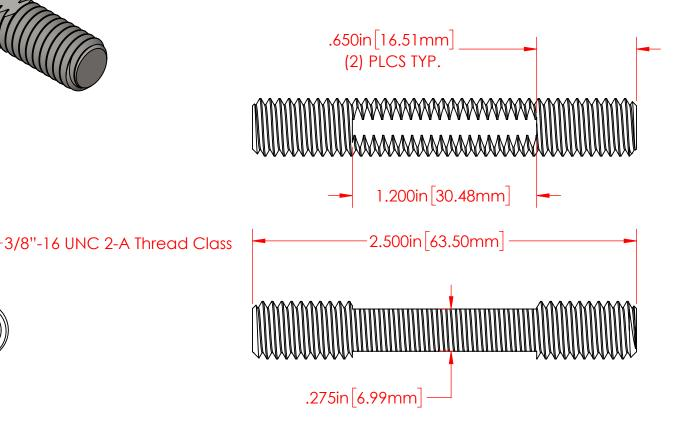
P/N 3755-000 Made from P/N 3742-011 3/8"-16 Threaded Stud Nickel Plated Mild Steel
