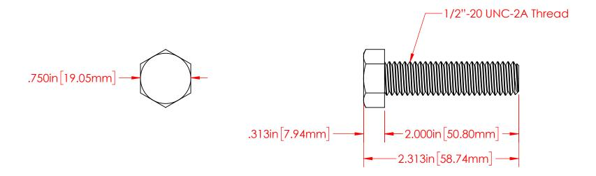
P/N 3757-001 1/2"-20 Fully Threaded 18-8 Stainless Steel Bolt
