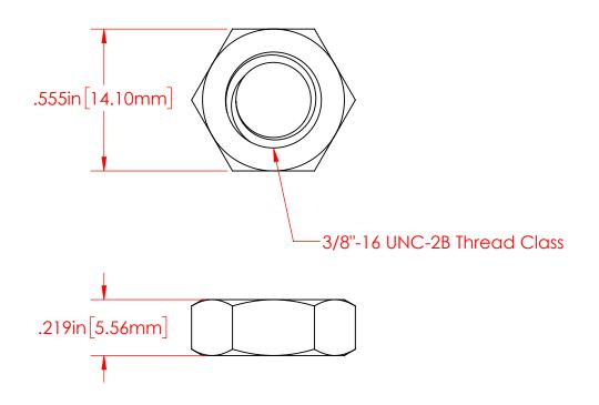
P/N 3838-000 3/8"-16 Brass Jam Nut 270 Brass Alloy
