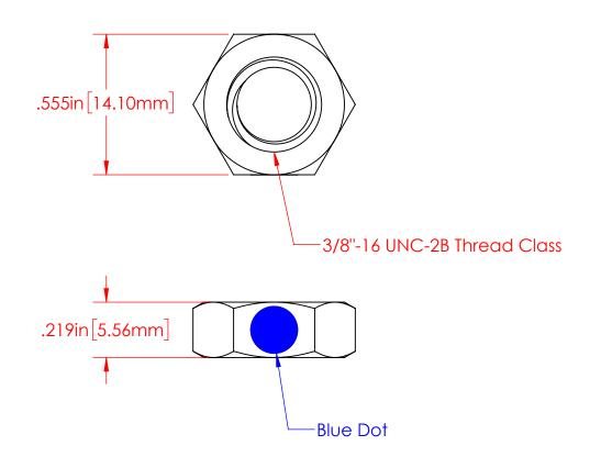
P/N 3838-B00 3/8"-16 Brass Jam Nut 270 Brass Alloy
