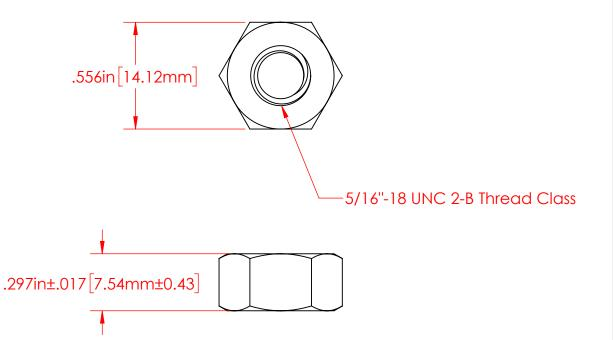
P/N 3843-003 5/16"-18 Heavy Hex Jam Nut Tin Plated 360 Brass Alloy
