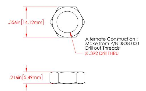
P/N 3843-X10 3/8" Jam Nut No Thread 360 Brass Alloy
