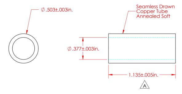
P/N 3863-000 Copper Core Bushing 122 Copper Alloy Annealed Soft
