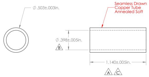
3864-000 Copper Core Bushing 122 Copper Alloy Annealed Soft
