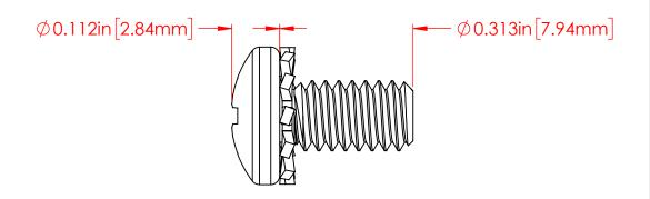
P/N 3870-000 Stainless Steel 8-32 x 5/16" Phillips Sems Screw with External Tooth Lock Washer
