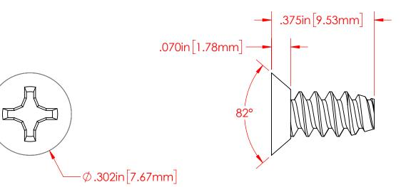
P/N 3874-000 Stainless Steel #8-18 x 3/8" Flat Head Uniform Thread Screw
