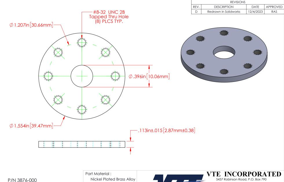
P/N 3876-000 Nickel Plated 360 Brass Alloy 8 Point Power Post 3/8" Contact Distribution Disk
