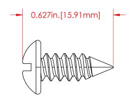
P/N 3880-000 #10 x 1/2" Combo Pan Head Sheet Metal Screw Zinc Plated Steel
