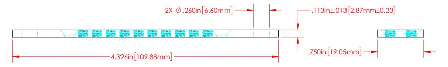
P/N 3886-000 Nickel Plated 360 Brass Alloy 10 Point Bus Bar Plate
