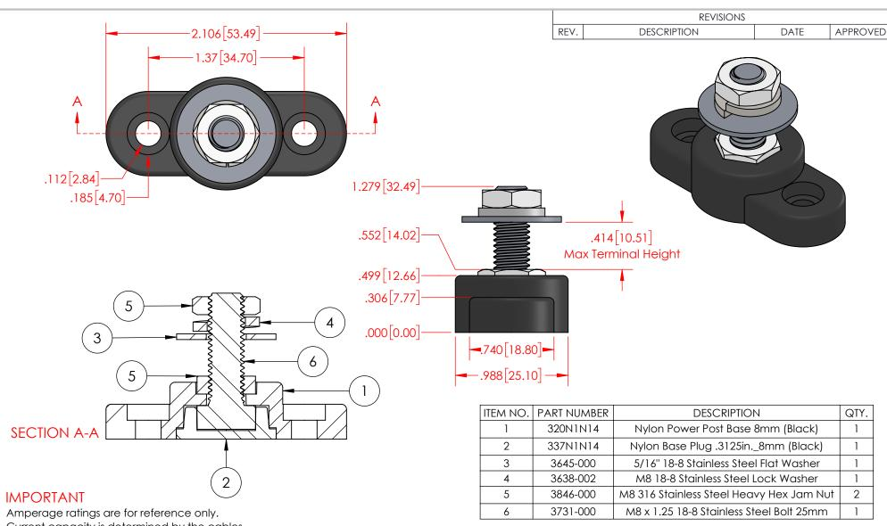
Current capacity is determined by the cables used, not the junction post. Current ratings are related to expected cable capacities.
