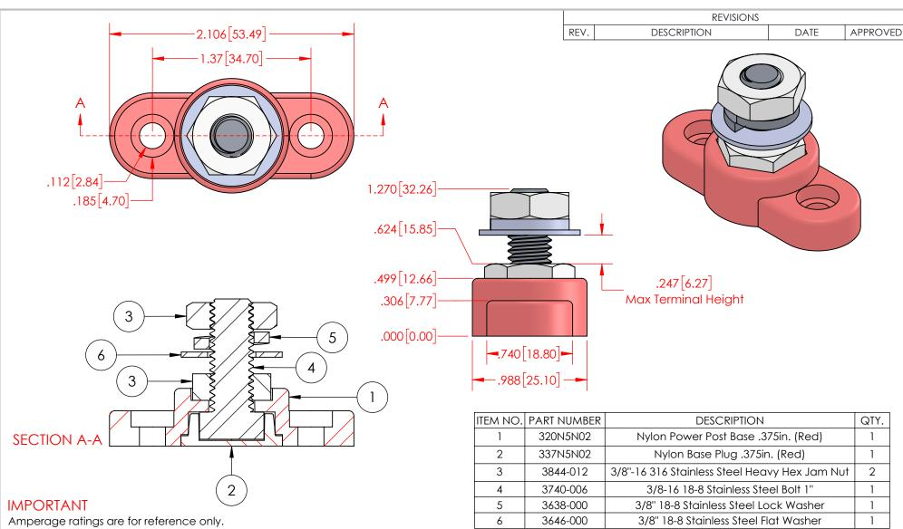
Current capacity is determined by the cables used, not the junction post. Current ratings are related to expected cable capacities.
