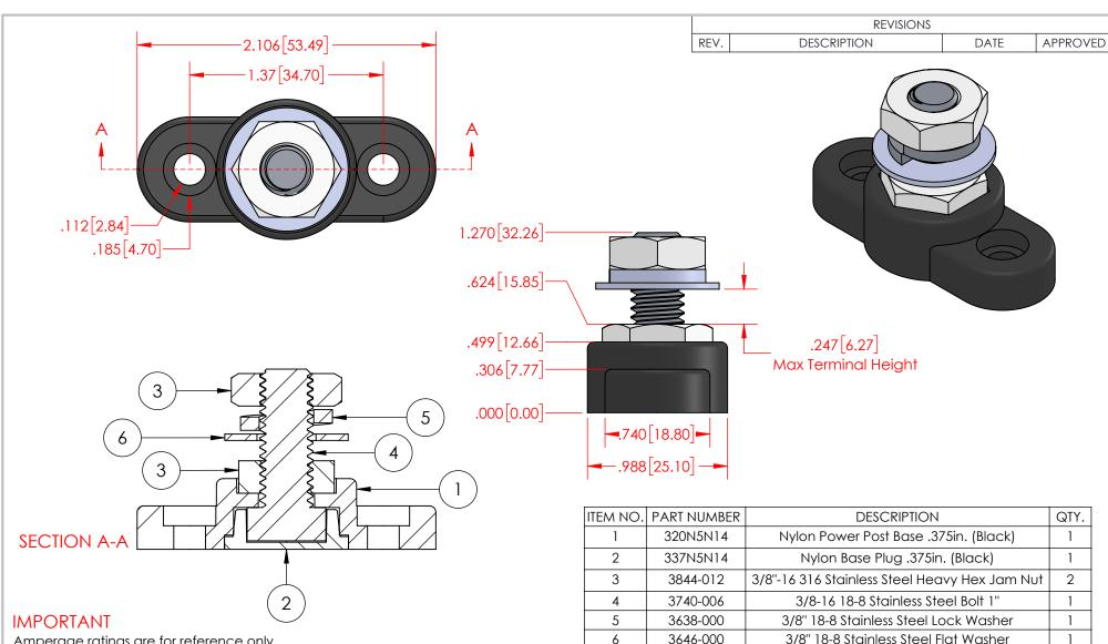
Amperage ratings are for reference only. Current capacity is determined by the cables used, not the junction post. Current ratings are related to expected cable capacities.
