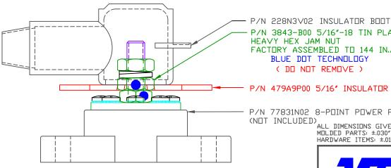
P/N 3843-B00 5/16"-18 TIN PLATED BRASS HEAVY HEX JAM NUT FACTORY ASSEMBLED TO 144 IN./LBS
