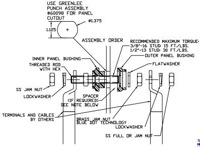
NOTE: IF INNER PANEL BUSHING DOES NOT PROTRUDE THROUGH PANEL BY 1/16", USE OF SPACER IS RECOMMENDED TO PREVENT DAMAGE TO OUTER PANEL BUSHING.
