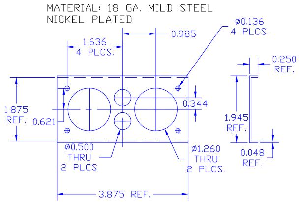
TOLERANCE UNLESS OTHERWISE SPECIFIED: HARDWARE ITEMS: ±.010"/±0.25mm RADIAL DIAMETERS TO BE MEASURED OVER MANDRELS, RING GAGES OR PIN GAGES OF SUITABLE SIZE
