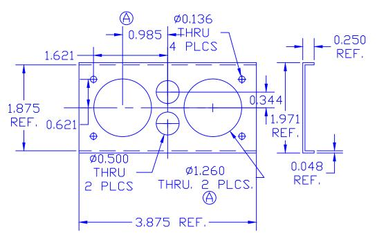
TOLERANCE UNLESS OTHERWISE SPECIFIED: HARDWARE ITEMS: ±.010"/±0.25mm RADIAL DIAMETERS TO BE MEASURED OVER MANDRELS, RING GAGES OR PIN GAGES OF SUITABLE SIZE
