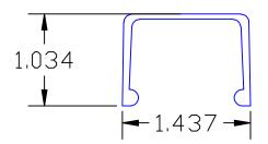
TOLERANCE UNLESS OTHERWISE SPECIFIED: ±.030"/±0.8mm RADIAL DIAMETERS TO BE MEASURED OVER MANDRELS, RING GAGES OR PIN GAGES OF SUITABLE SIZE
